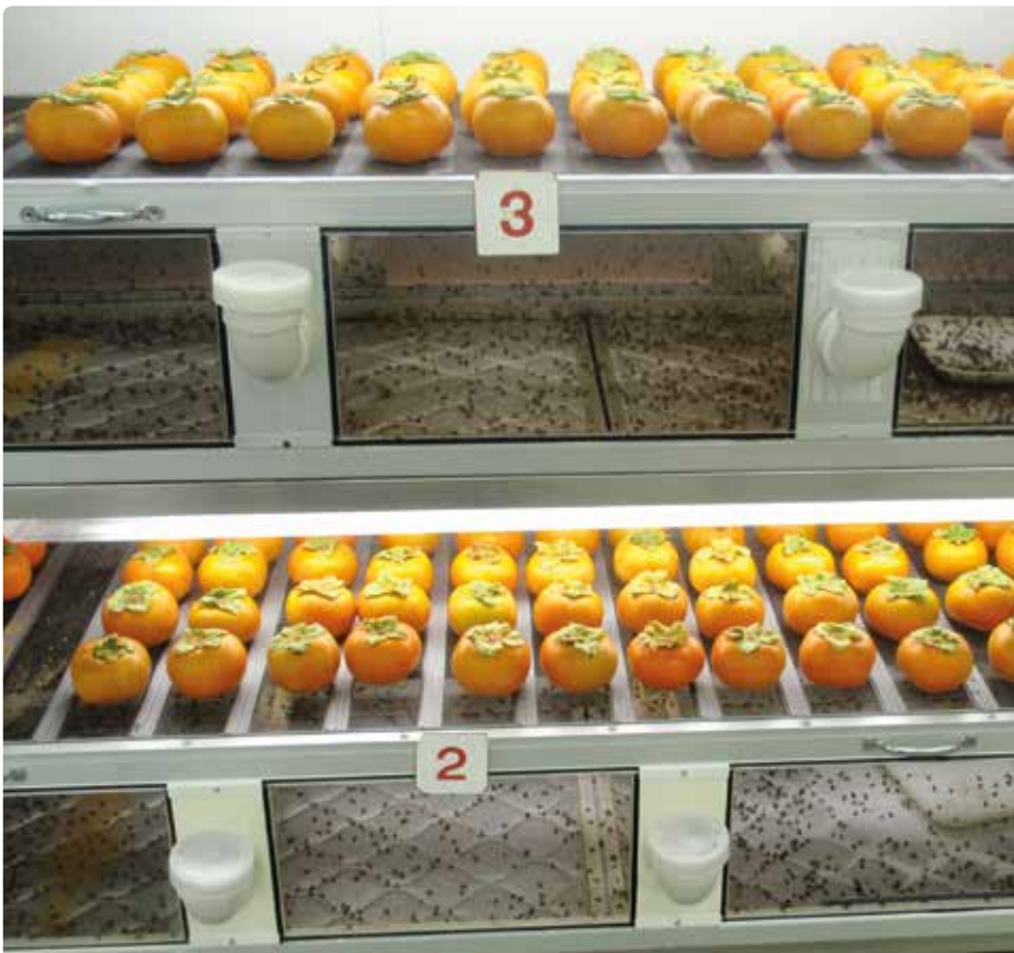
Infesting Fuyu persimmons with QFF at a New South Wales Department of Primary Industries disinfestation trial
